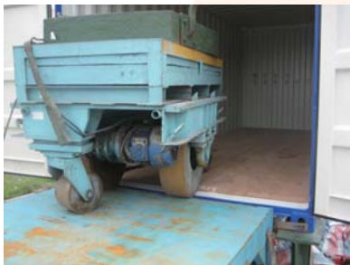
7,260kg loading test for Brigantine container floorboards
