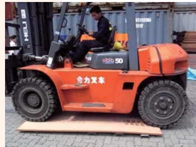
Simulated loading test by 8 tons forklift by our Storekeeper in IQC program
